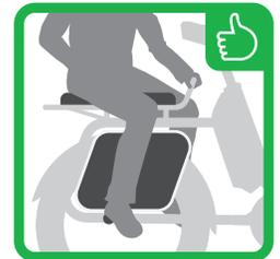
**WHEN CARRYING PASSENGERS, REAR WHEEL MUST BE COVERED! INSTALL BENNO REMIDEMI WHEEL GUARDS, SEAT PAD AND FOOT PEGS. FAILURE TO DO SO COULD RESULT IN SERIOUS INJURY!** MAKE SURE THAT NO PARTS OF THE BODY OR CLOTHING COME NEAR MOVING PARTS ON THE BICYCLE, SUCH AS CHAIN, SPOKES, TIRES OR BRAKES. DO NOT EXCEED TOTAL MAX GROSS WEIGHT OF THE BIKE AND/OR RACK MAX LOAD.
