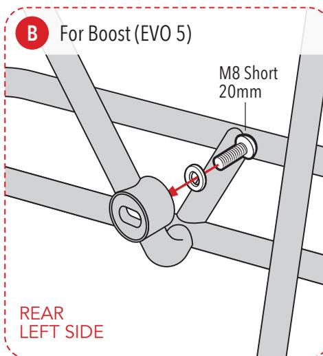
**REAR LIGHT PLATE: DISASSEMBLE EXISTING LIGHT PLATE THEN REASSEMBLE WITH NEW RACK IN PLACE**
