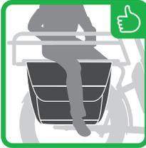
**WHEN CARRYING PASSENGERS, REAR WHEEL MUST BE COVERED! INSTALL BENNO WHEEL GUARDS OR UTILITY PANNIER BAGS. FAILURE TO DO SO COULD RESULT IN SERIOUS INJURY!** MAKE SURE THAT NO PARTS OF THE BODY OR CLOTHING COME NEAR MOVING PARTS ON THE BICYCLE, SUCH AS CHAIN, SPOKES, TIRES OR BRAKES. DO NOT STAND ON SIDELoadERS. MAX SIDE LOAD IS 15KG/35LB EACH SIDE. HOWEVER, COMBINED RACK LOAD (DECK+SIDES) NOT TO EXCEED 60KG/130LB. FASTEN CARGO SECURELY AND MAKE SURE ALL STRAPS AND HOOKS ARE TIGHTENED.
